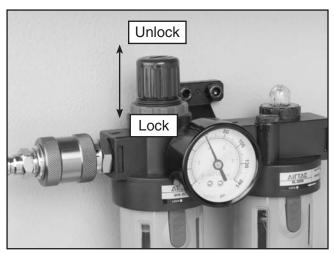
**Figure 17.** Air pressure regulated to 60 PSI at the gauge.
